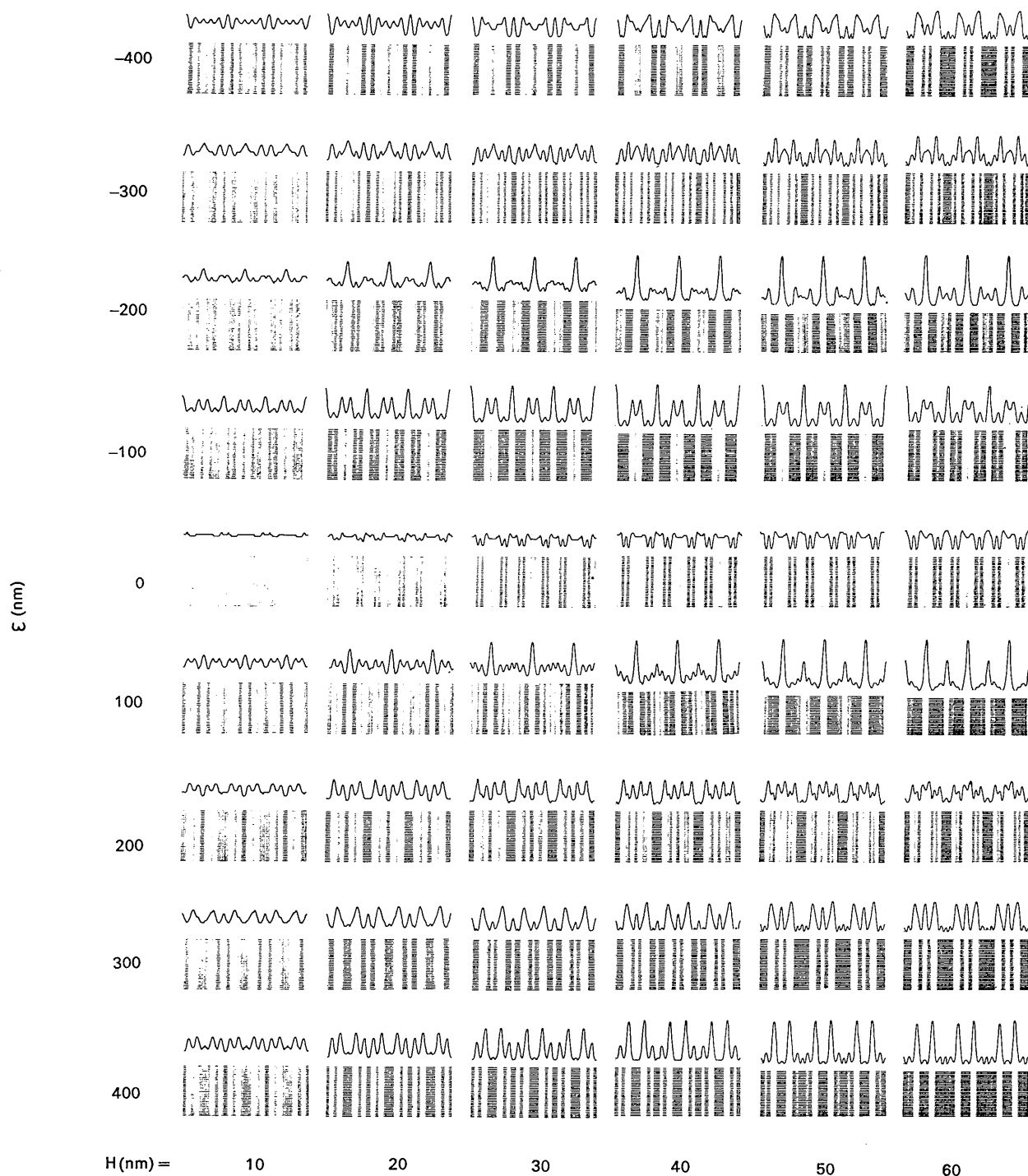
Fig. 7. Image contrast for a range of defects of focus ranging from -400 nm at the top of the display to +400 nm at the bottom in steps of 100 nm. The columns are arranged for crystal thicknesses ranging from 10 nm to 60 nm in steps of 10 nm from left to right. The calculations are from the 435 reflexion two-dimensional multislice method. There is only a small variation in image contrast as a function of crystal thickness.
